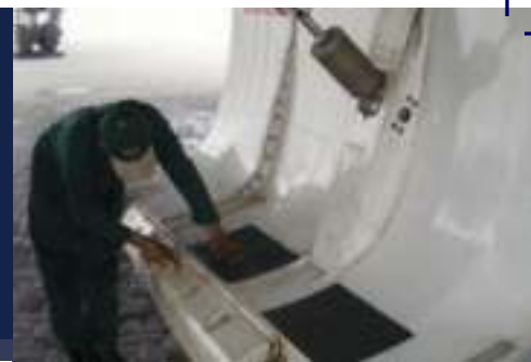
747 Landing Gear Door Cleaned With eOx
